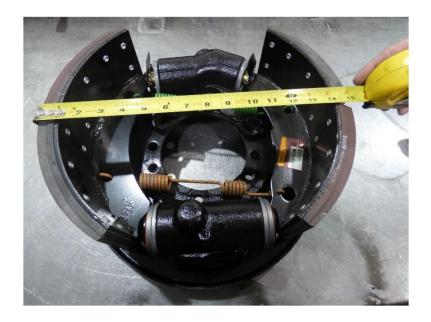
3. When installing the shoes, use the proper tool to insure that you do not cut the boots and cause a premature failure and void the warranty.
