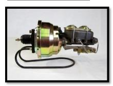
The perfect solution for many vehicles. A complete, modern brake system which is available in a 7" or 8" double diaphragm booster (bigger is better if you have the room), low profile dual bail master cylinder with line attachments on either side (opposite side is plugged), bracket to attach the included proportioning valve which is either a PV2 (disc/drum) or PV4 (disc/disc) proportioning valve depending on the vehicles current configuration.
