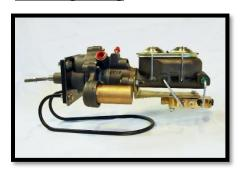
\*\*Note: this unit requires a power steering pump to operate. Additional fitting may be needed on power steering pump depending on vehicle.
